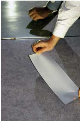
Image 2: Apply the Gellifter so that the center-point of each end covers one of the laser dots.
